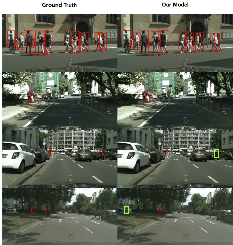
Fig. 5 Exemplar detections of our proposed SASR-CSP on Citypersons dataset. The first column is the ground truth. The red bounding box represents the correct detection. The green bounding box represents the miss detection. It can be seen that our proposed model performs well at different occlusion levels. The crowded pedestrians and small pedestrians can be detected accurately. Some heavily occluded pedestrians are missing
