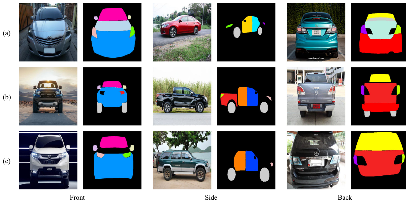
Fig. 8 Samples of pair images and instance mask from the DSMLR Car Part data set: a sedan, b pickup and c sports utility vehicle (SUV)
