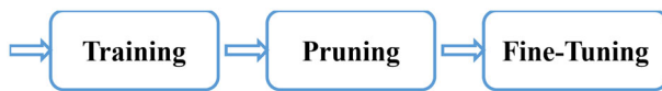
Fig. 1 A typical three stage pruning pipeline. A network is first well trained in a target dataset, and then the pre-trained model is pruned with certain method. After pruning, the pruned model is fine-tuned, in which the model is retrained with lower learning rate on the dataset
