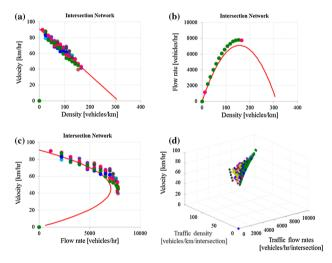
Fig. 12 Collecting plot of all traffic relationships of the intersection network, compared with the Greenshields model (a). Traffic velocity and traffic density (b). Traffic flow rate and Traffic density (c). Traffic velocity and traffic flow rate and (d). Triple plot of all traffic parameters
