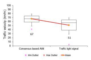
Fig. 16 Comparison plot of traffic velocity between traffic light signal and consensus-based AIM
