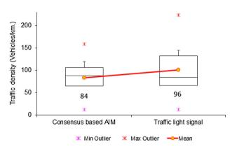
Fig. 17 Comparison plot of traffic density between traffic light signal and consensus-based AIM
