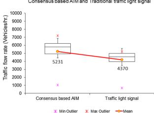
Traffic flow rate in the intersection network between Consensus based AIM and Traditional traffic light signal
