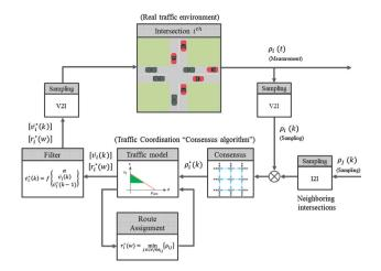
Fig. 19 Closed loop control block diagram of an intersection manager with the route assignment
