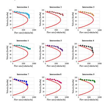
Fig. 10 The comparison of traffic velocity and the traffic flow rate relationship of each intersection in the network
