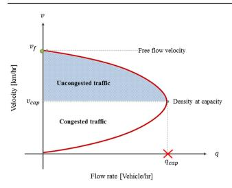
Fig. 5 Relationship between velocity and flow rate
