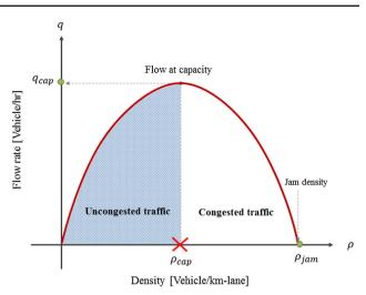
Fig. 4 Relationship between flow rate and density
