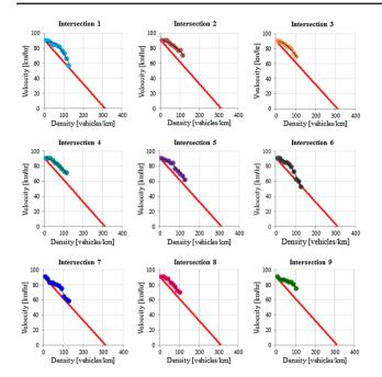
Fig. 9 The comparison of traffic velocity and the traffic density relationship of each intersection in the network
