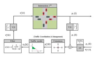
Fig. 7 Closed loop control block diagram of an intersection manager
