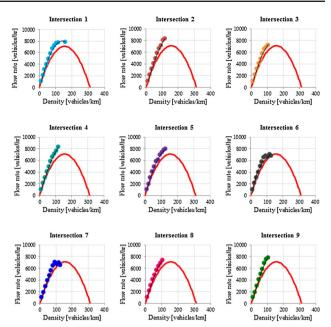
Fig. 11 The comparison of traffic flow rate and the traffic density relationship of each intersection in the network
