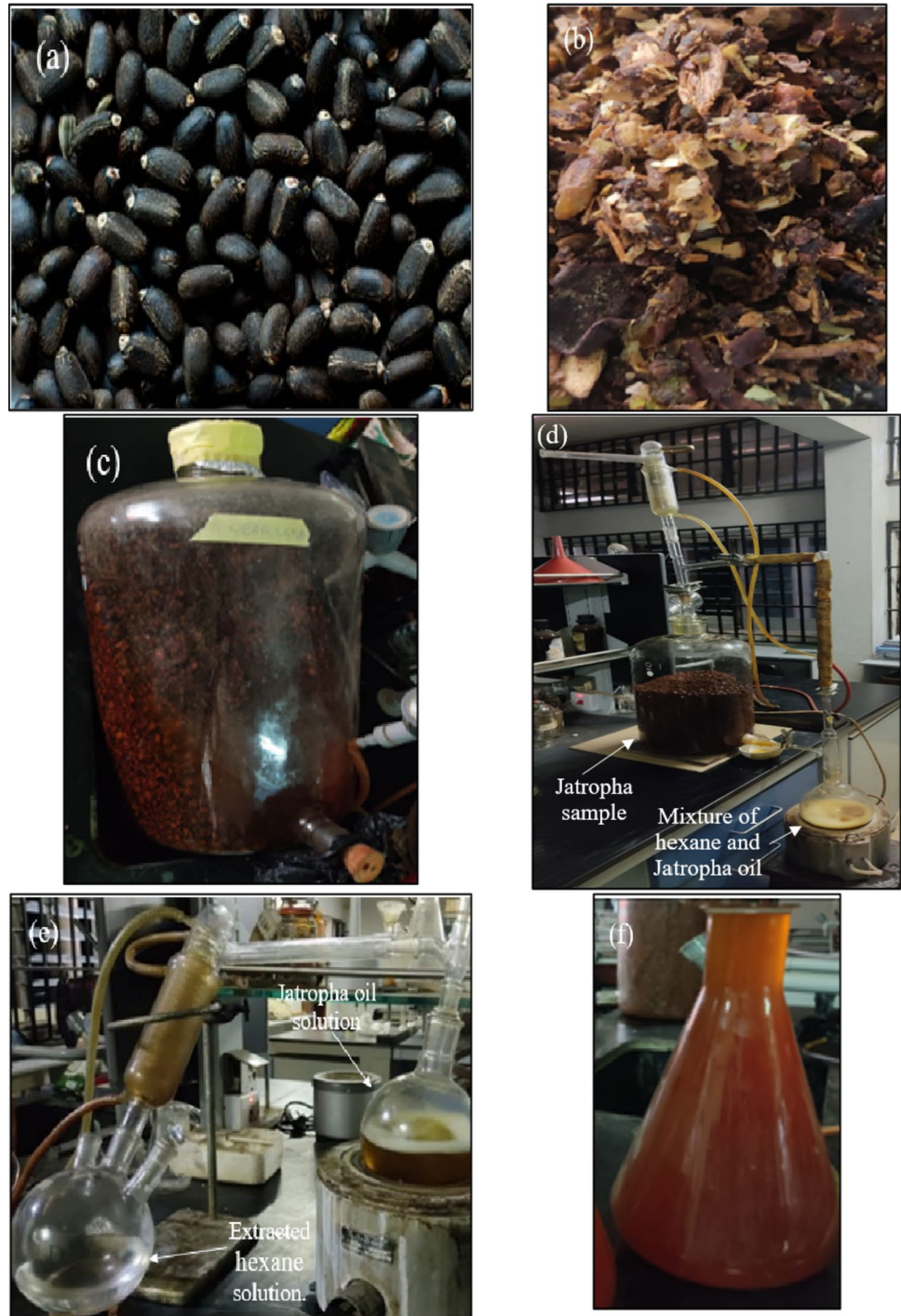
Fig. 1 Photographic views of the extraction process. (a) Dry jatropha seeds; (b) Milled jatropha seeds; (c) Milled seeds in the beaker before extraction; (d) Jatropha oil extraction; (e) Distillation process to separate hexane from extracted oil; and (f) Crude jatropha oil after extraction
