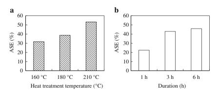
**Fig. 1** Anti-swelling efficiency (ASE) of heat-treated wood at different treatment temperatures (**a**) and at different treatment times (**b**). Data adapted from [109]
