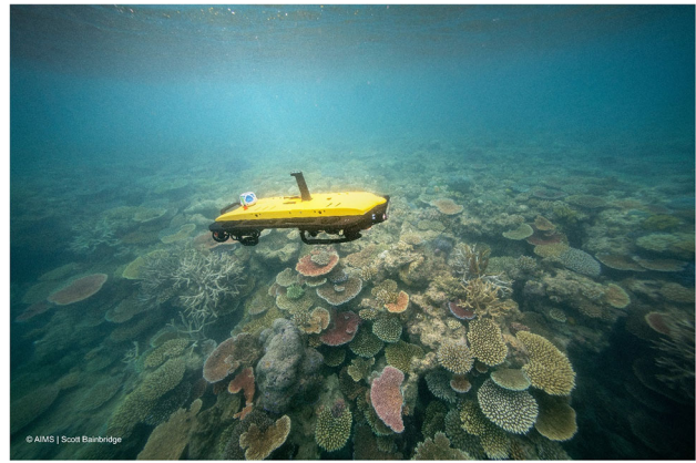
Fig. 4 CoralAUV Platform (Australian Institute of Marine Science 2023)
