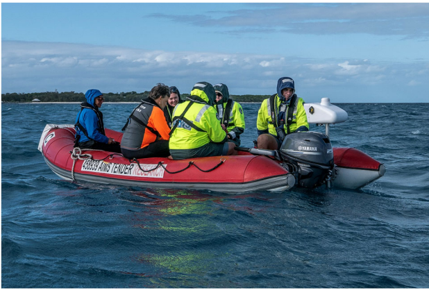
Fig. 3 The transom-mounted ReefScan system (Australian Institute of Marine Science 2023)
