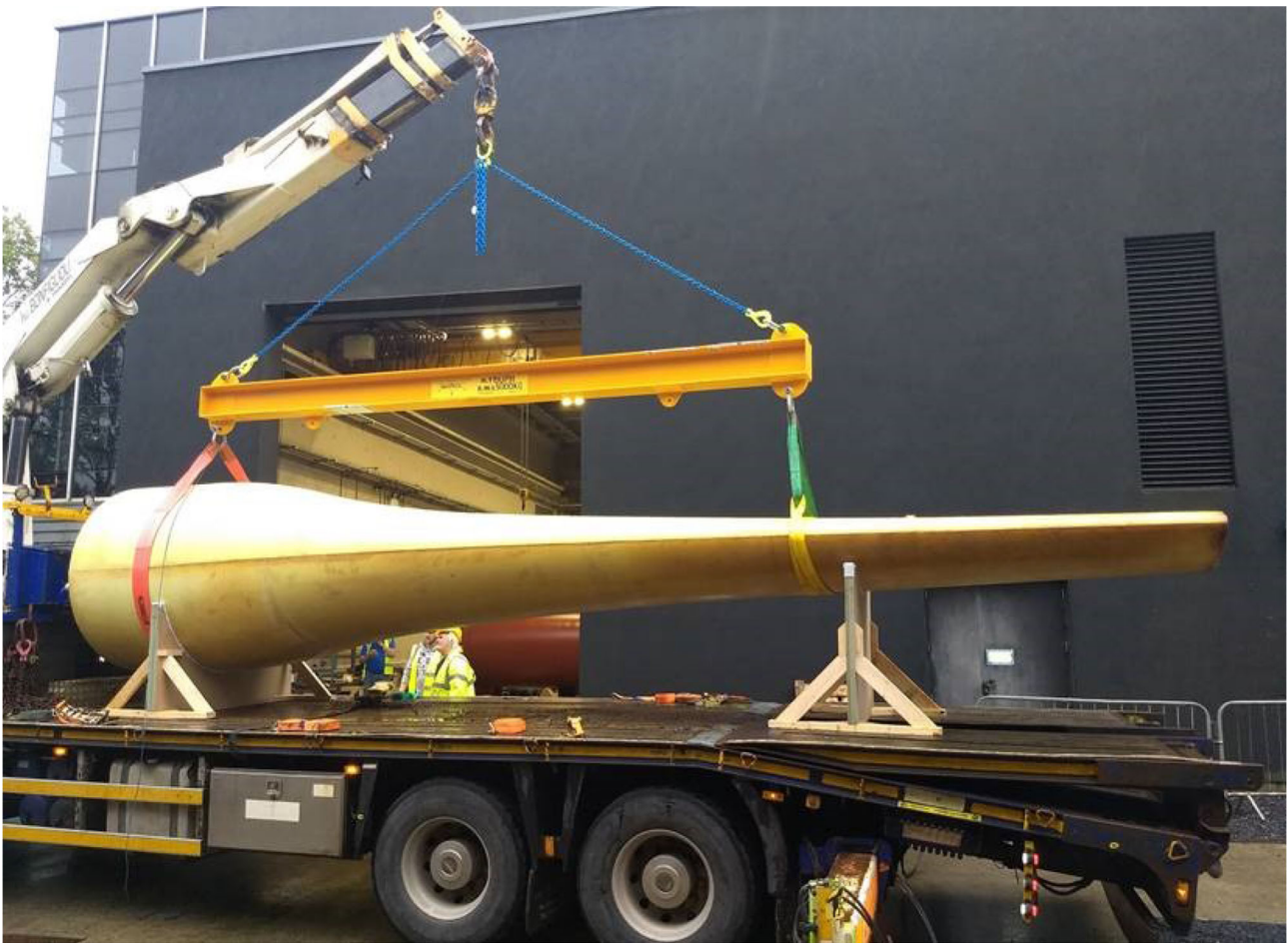
Fig. 1 The 1-MW tidal turbine blade (manufactured at ÉireComposites)
