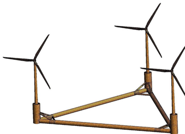
Fig. 3 The shell elements of the wind-tracing FOWT and the turret
