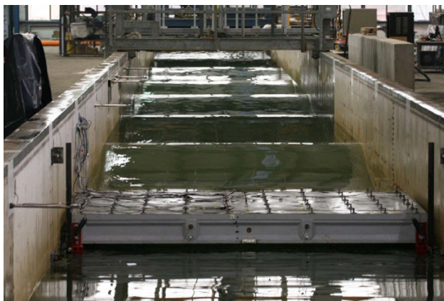
Fig. 2 Experimental setup to measure wave forces on a coastal bridge (Bradner 2008)
