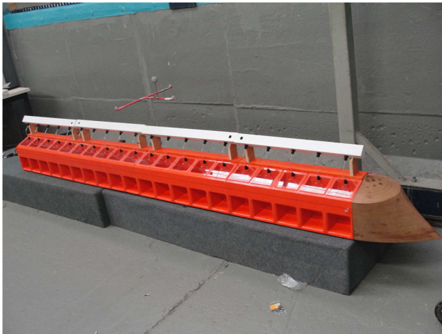
Fig. 11 Photo of the scale model ready for testing. A removable bow section is fitted in this picture, but results are presented here only without the bow
