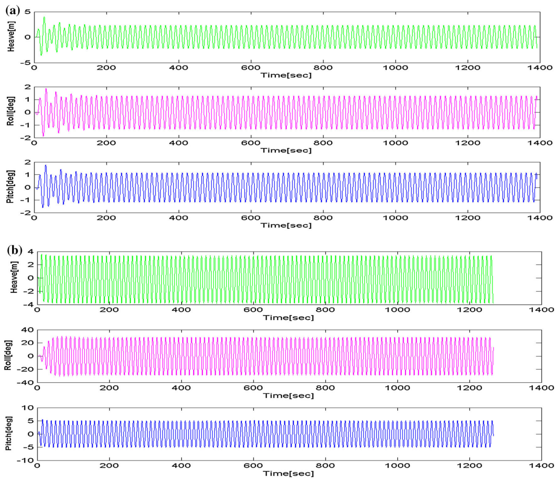
Fig. 4 Time-histories of the motion responses from the fully linearized algorithm. a Semisubmersible motions for wave period ( T ) = 14 s, wave height ( H_w ) = 12 m, wave heading ( \beta ) = 135°. b S175 hull motions for T = 12 s, H_w = 10 m, \beta 135°
