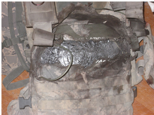
Fig. 3 A soldier suffered no significant injury after being struck in his chest wall body armor by a rocket-propelled grenade. (Photo courtesy of COL Matthew Martin)
