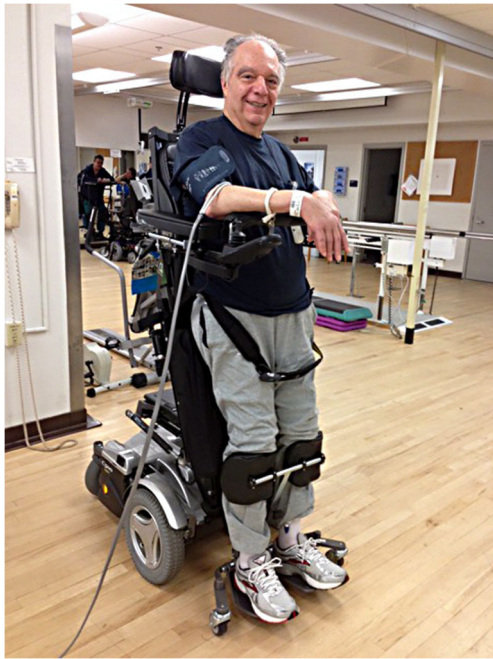
Fig. 3 Patient in standing frame with abdominal belt (loose) and tibial support. (Courtesy of Nancy Kelly)
