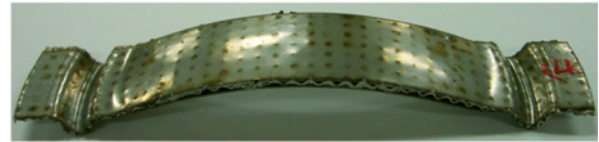
Fig. 13 Example of the stretch formed thin metallic sandwich plate with dimple inner structures (reprinted from figure provided by Prof. Dong-Yol Yang, Prof. Jong-Ho Kim and Dr. Dae-Yong Seong with permission)
