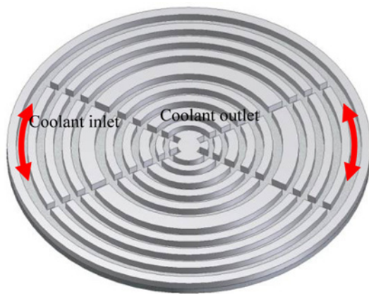
Fig. 9 Circular shaped platen coolant channels
