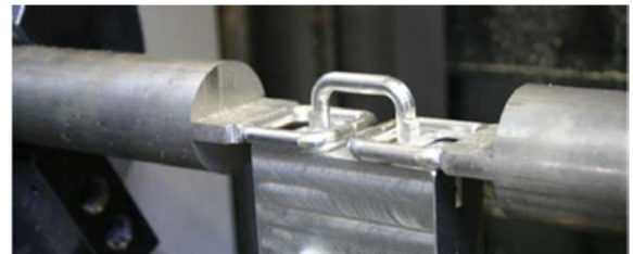
(a) Clamping of the middle ring
