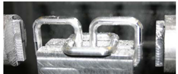
(b) Separation of rings from support
