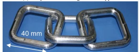
(c) Finished chain-shaped ring
