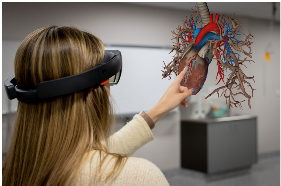
Fig. 1 An example of the participant experience when learning through the mixed reality device. The 3D model is visible in front of the user, with hand gestures and voice commands allowing interactivity, while the lesson plays as an audio stream through the headphones
