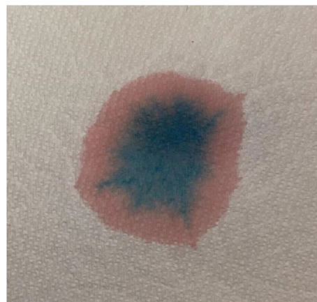
Fig. 2 Color chromatography demonstrating separation of red and blue components
