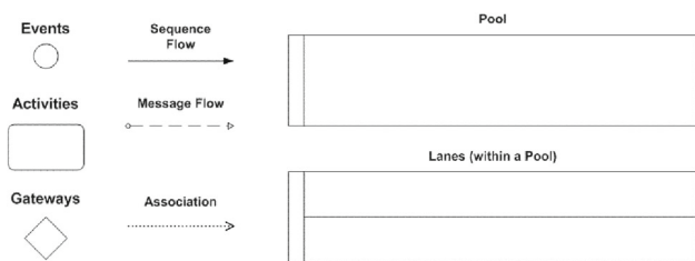
Fig. 5 Core subset of BPMN elements
