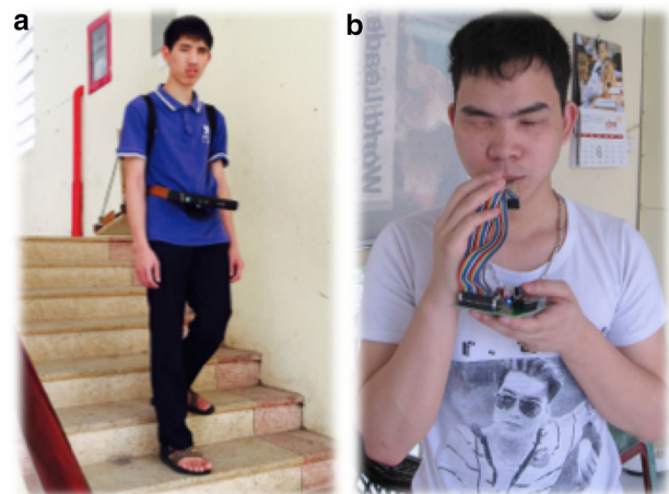
Fig. 14 Illustration of the warning device. a Kinect sensor on user and b control module and electrode matrix on user. a Kinect sensor mounted on the belt worn by a blind student. Video processing is conducted by a laptop placed on a backpack. b The tongue electrotactile device worn on a blind user. The matrix of electrodes is place totally inside the mouth in contact with the dorsal part of the tongue and is controlled by the module through cables
