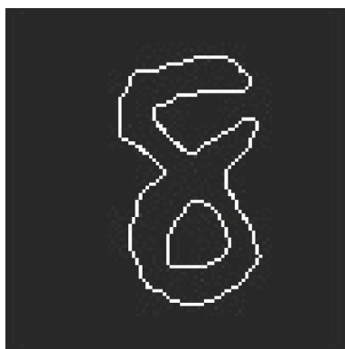
Fig. 9 Boundary pixel image from size normalized binary image
