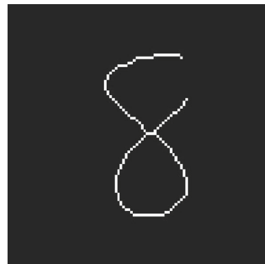
Fig. 8 Skeleton image from size normalized binary image
