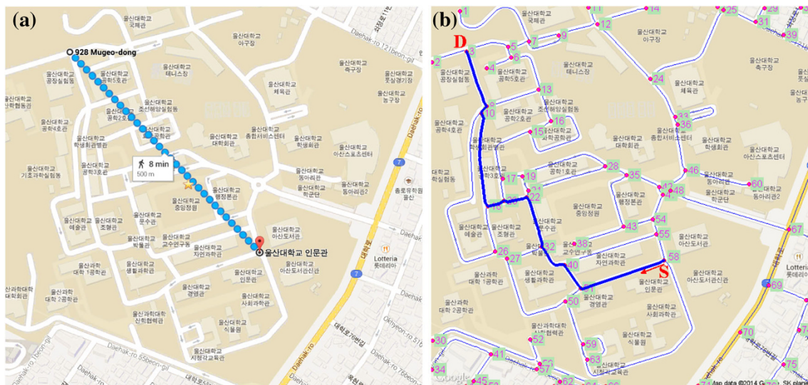
Fig. 13 The shortest path estimation a Google result, b our proposed method estimated result from the source S to the destination D , of road network (denoted by light-blue) and the shortest path (denoted by thick blue)
