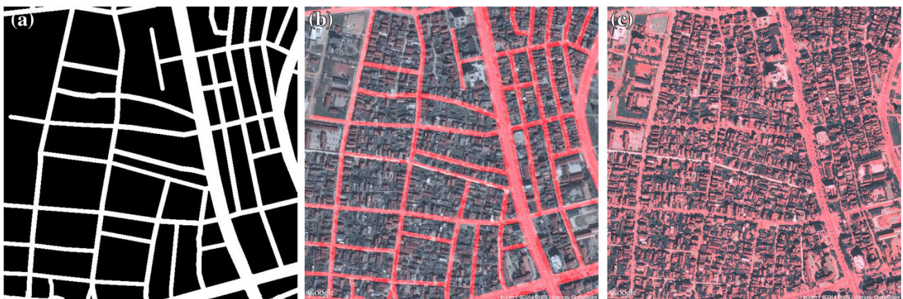
Fig. 7 Color filter a road region result from road map layer, b corresponding road regions in terrain layer (annotated by light-pink ) to learn color model for detection, c road candidate regions (annotated by light-pink ) using color detection
