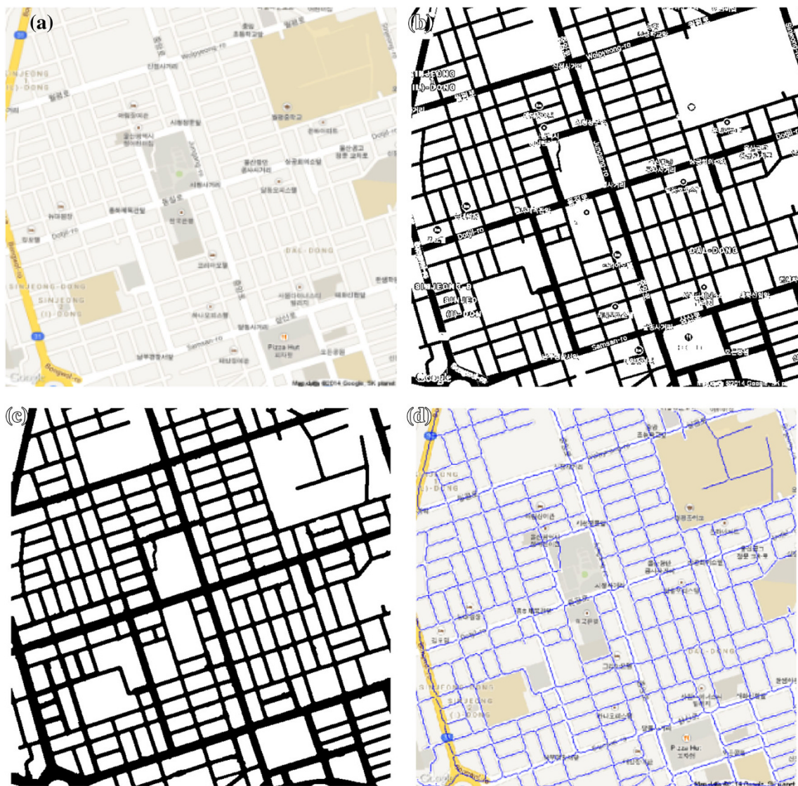
Fig. 5 Path-network detection a road maps image, b road candidates are estimated by color filter and segmentation, c post process to connect the discontinuous road regions, d path network extraction
