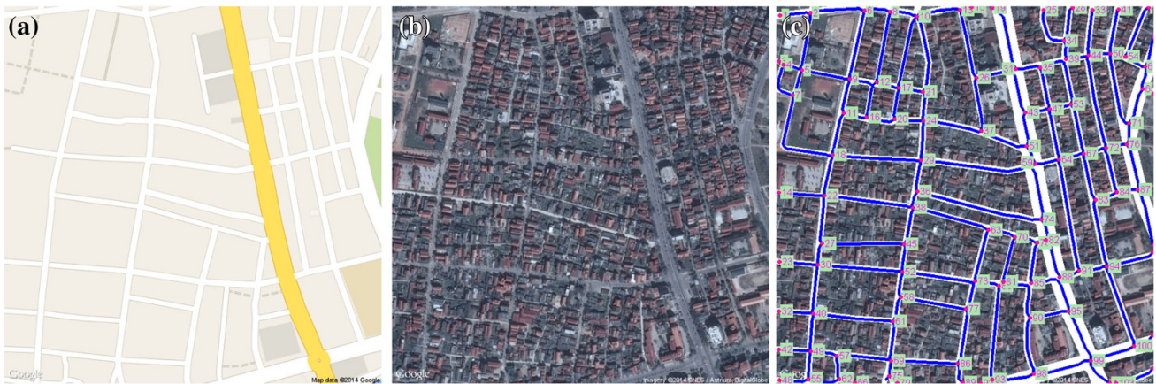
Fig. 6 Some road segments are not marked by services a road map image, b satellite image, c road network detection using both of GIS layers
