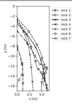
**Fig. 13** Path of the impacting rocks. The ordinate y[m] depicts the vertical, gravitational direction. The abscissa z[m] visualizes the out-of-plane direction of the protection net. Y=0 at the top position of the construction
