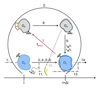
Fig. 9 General FSI strong coupling algorithm diagram
