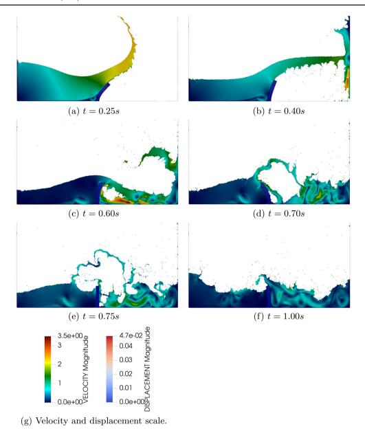
Fig. 17 Collapse water column against an elastic structure. Numerical results at different time instants. The velocity contours are plotted over the fluid mesh
