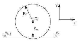
(a) DEM particle contact detection with edge spanning between node  $v_{k-1}$  and node  $v_k$ , adapted from Santasusana et al (2016); Sautter et al (2021c)
