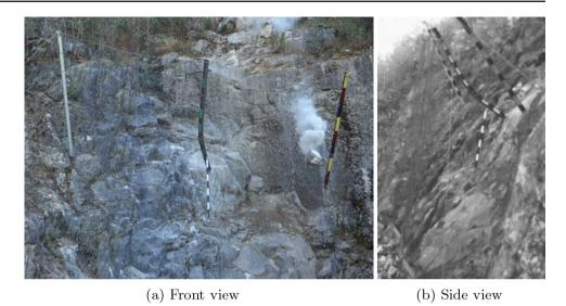
Fig. 12 Multiple rocks simultaneously impact the attenuator structure. The protection structure guides the impacting rocks to a safe zone
