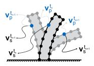
(b) Velocities of the particle and structure in the coupled case
