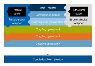
Fig. 4 Minimal modular coupling scheme representation
