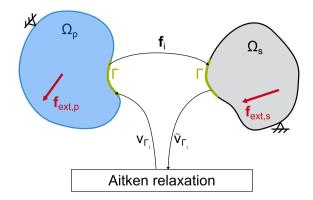
Fig. 8 Aitken relaxation diagram, adapted from [11]
