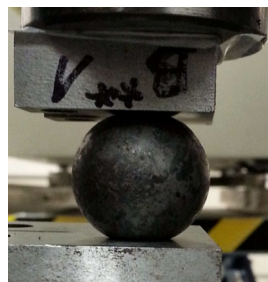
Fig. 4 Balls used for the tests: with diameters of 30 mm, 40 mm, and 50 mm
