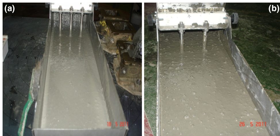
Fig. 1 Filling and passing ability of SCC Mix 1 (a) and Mix 2 (b)
