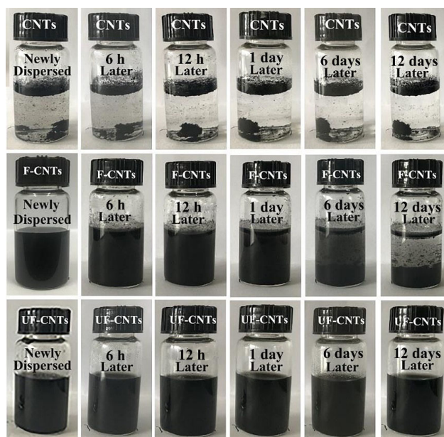
Fig. 23 Dispersion properties of 0.15 wt% CNTs, 0.15 wt% F-CNTs, and 0.15 wt% UFCNTs in the water. Reproduced with permission from Ref. [140], © Elsevier 2019.
