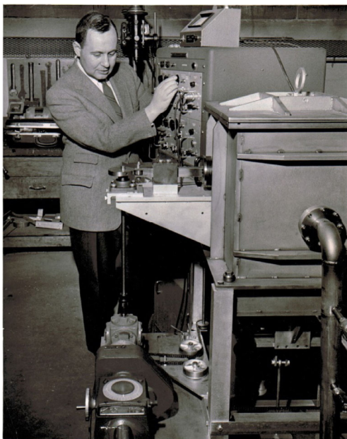
Fig. 1 Ernest Rabinowicz “hard at work”. On this photo taken in the late 1950s or early 1960s he is absorbed in work with a cylinder on cylinder rolling tester [10].
