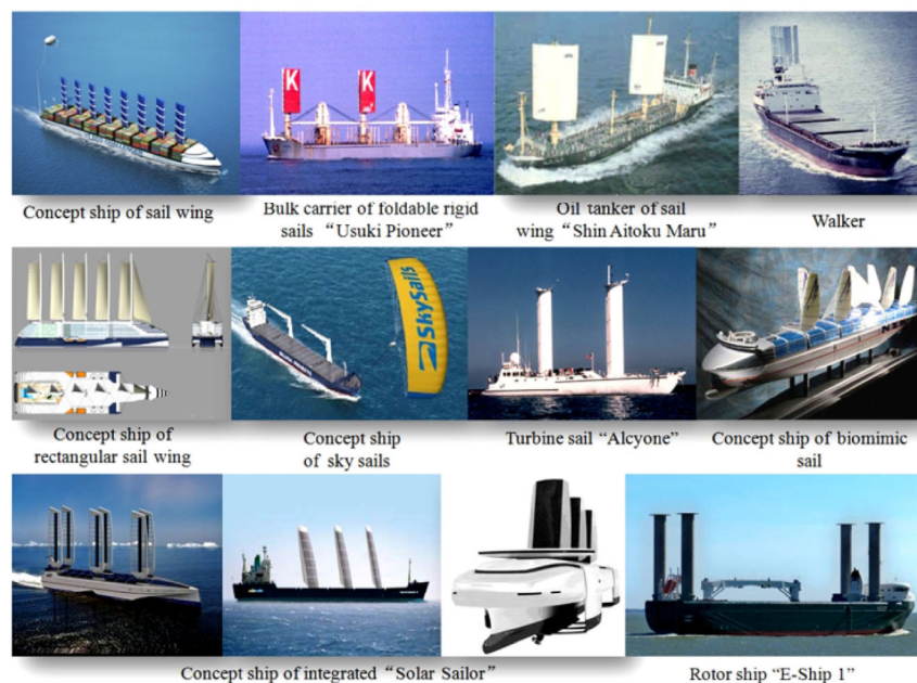
Fig. 4 Various types of sail-auxiliary ships.
