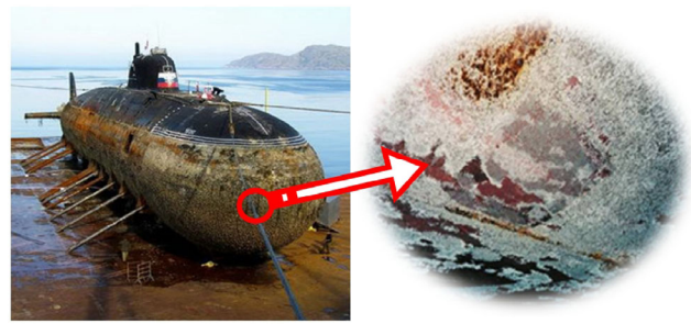
Fig. 10 Fouling and corrosion on the hull surface.
