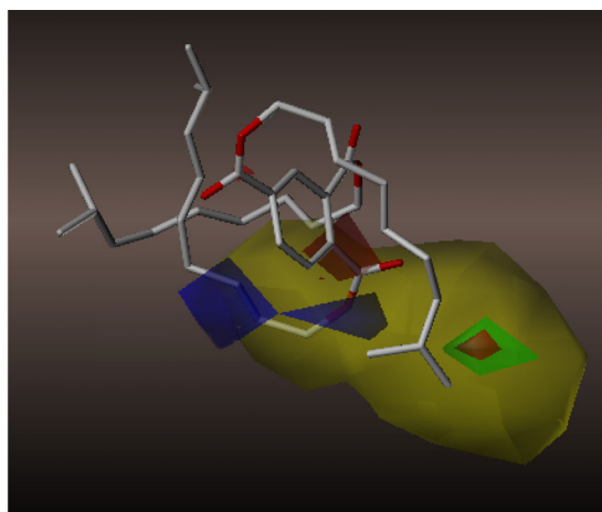
Fig. 39 CoMSIA contour diagram for wear with embedded triisodecyl trimellitate as reference for both steric and electrostatic fields. Green and yellow regions show where steric bulk is favored and disfavored, respectively. Blue region shows where positive charge is favored while red region shows where negative charge is favored.
