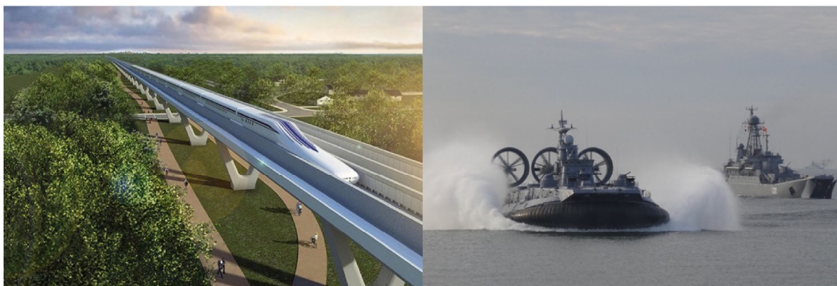
Fig. 3 Maglev train and hovercraft move frictionlessly because of the interface magnetic repulsion force and the air ejection (Public domain).
