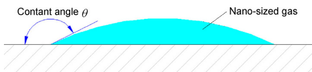
Fig. 3 Nanosized gas at water–solid interface.
