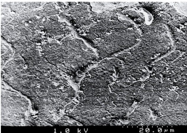
Fig. 5 A close-up of the perpendicular ridges occurring at locations of highest tractive force at the tibial plateau.
