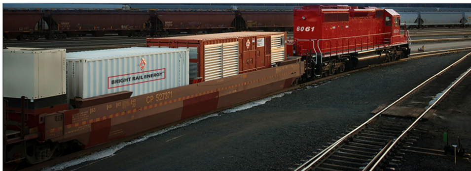
Fig. 4 Locomotive and trailing car arrangement (carrying fuel heating generator, CNG storage container, and auxiliary power unit) used in Canadian Pacific – Bright Energy collaboration
