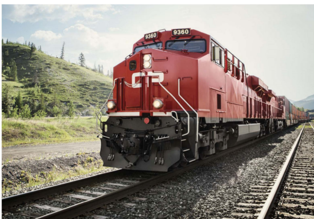
Fig. 1 Typical diesel-electric road locomotives (two head-end 3,275 kW AC units shown) in mainline usage on Canadian Pacific
