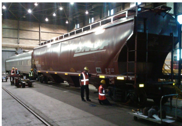
Fig. 10 A picture of the business car and the freight railcar being instrumented for the field test at the Transportation Technology Center, Inc. (TTCI)
