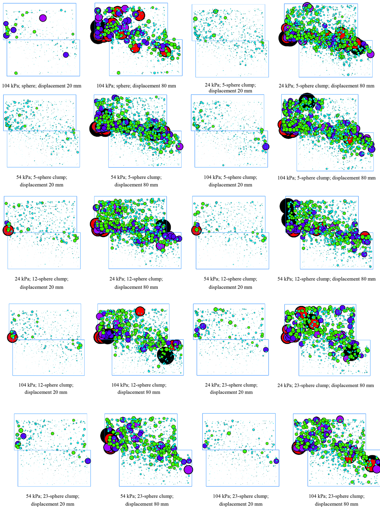
Fig. 16 Particle rotation illustration of the DST models
