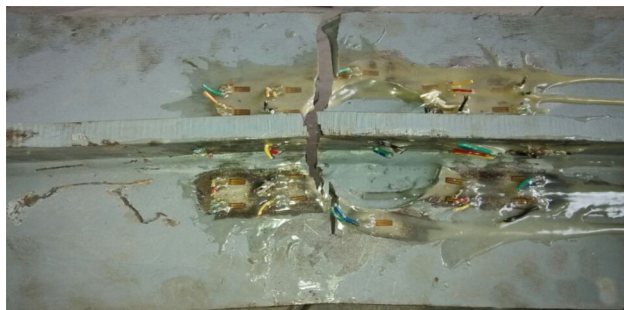
Fig. 3 Fatigue fracture of the specimen
