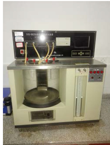
Fig. 2 Dynamic viscosity test device
