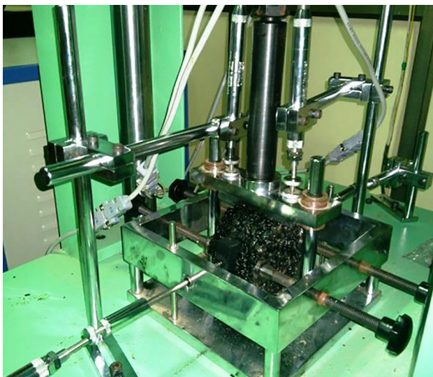
Fig. 6 Specimen arrangement in repeated load testing machine
