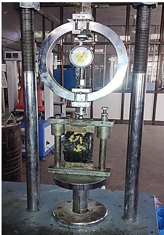
Fig. 2 ITS test setup
