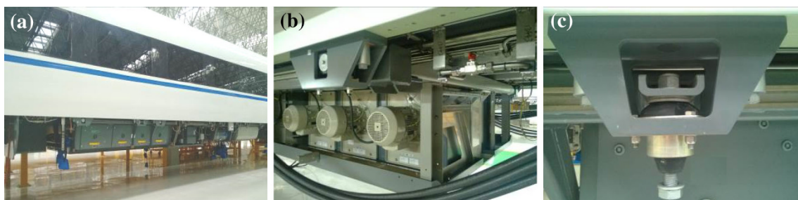
Fig. 1 The carbody of EMU: a suspended equipment under the chassis of carbody; b equipment with vibration excitation source; c rubber elements applied to connect the equipment to carbody elastically
