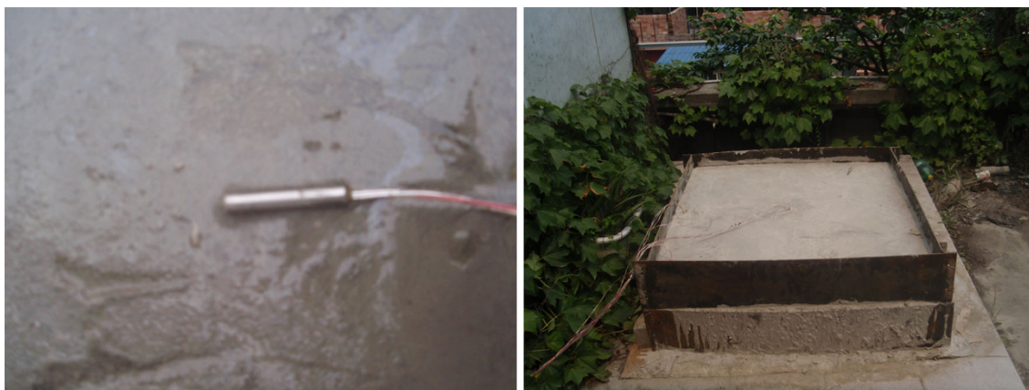
Fig. 2 The temperature sensors and the track slab for this test
