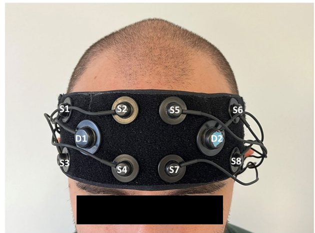
Fig. 1 Location of the OctaMon functional near-infrared spectroscopy (fNIRS) probe (Artinis Medical Systems; Netherlands) with 8 sources (1–8) and 2 detectors (D1–D2) covering the forehead of participants
