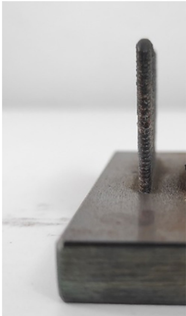
Fig. 10 Sample 2—Variable Wall Width
