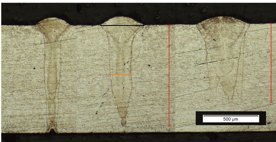
Fig. 5 Cross sections perpendicular to feed direction, P=400 W, d=40 \mu\text{m} , v_s=100 mm/s; left: a=0 , f=0 Hz; middle: a=80 \mu\text{m} , f=700 Hz; right: a=160 \mu\text{m} , f=700 Hz (width W_0 : black line, width W_{1/2} : yellow line, depth D : red lines)
