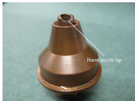
Fig. 10 Melted DMD nozzle due to back reflected light when using 3 kW laser power
