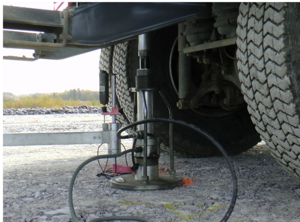
Fig. 1 Static PLT with 300-mm diameter plate and a truck as counterweight
