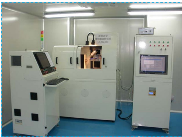
Fig. 27 Inclined axis magnetorheological polishing equipment [145]
