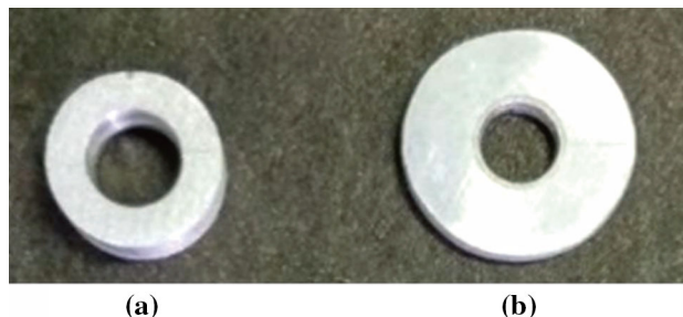
Fig. 5 Specimens before and after ring compression test a initial specimen, b specimen after compression
