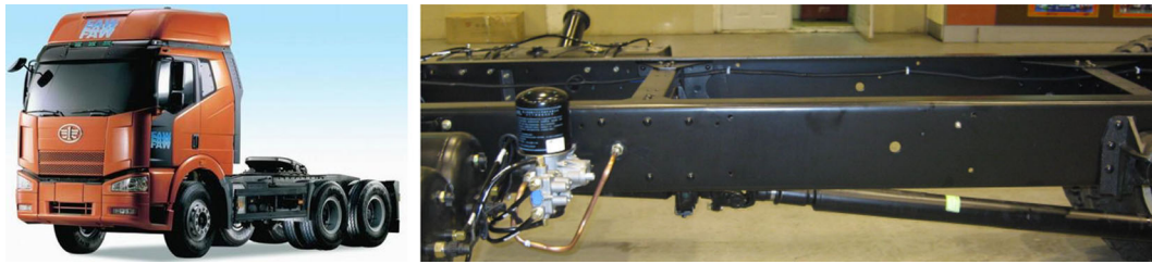
Fig.10 Weight reduction of 150 kg by using HSS in the frame structure (FAW)
