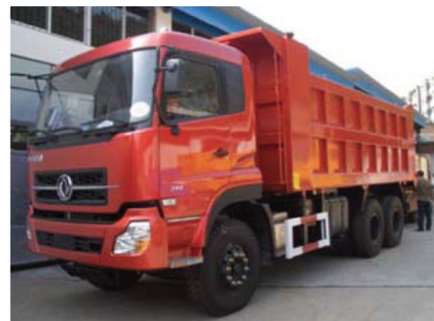
Fig. 9 Weight reduction of 250 kg in a dump truck by upgrading to D700L steel grade (Dongfeng)
