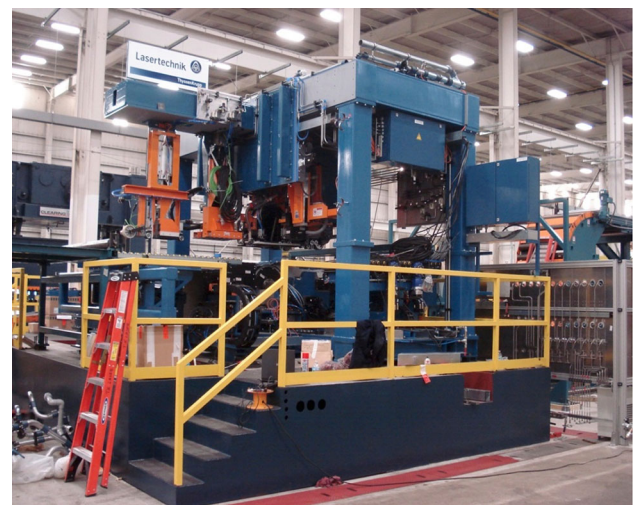
Fig. 17 Core unit with laser weld cell of an industrial tailor welded coil production line
